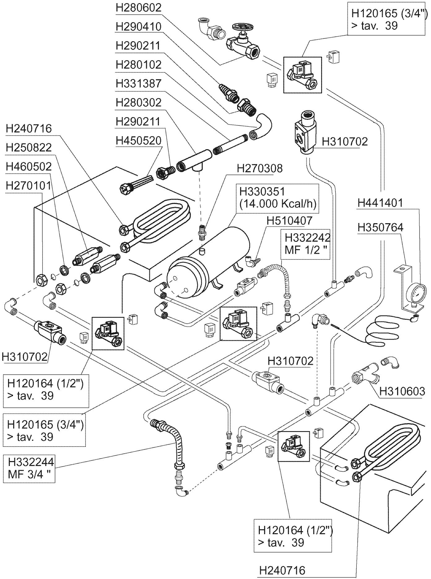
ELETTROVALVOLA VAPORE - ELECTROVANNE VAPEUR - STEAM SOLENOID VALVE - DAMPF-VENTIL- ELECTROVALVULA VAPOR
