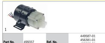
458552-01 LMP-20CPA magnetic-drive pump KITASHIBA type LMP-20CPA 17/20W 100V description 50/60Hz inlet ø 16mm outlet ø 14mm L 132mm
